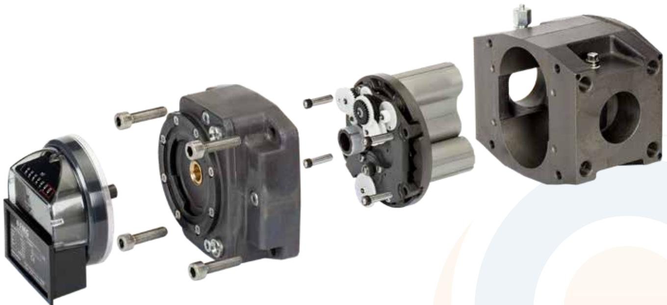
The use of a cartridge (pre-calibrated) and the accessibility of the front and rear bearings without the need for removing the timing gears, make the FMG series of rotary meter unique in terms of repair. Any repair shop can repair or re-condition the meters without special skills and tools. When regulation permits, a new, calibrated cartridge can be installed.
