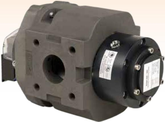
The most convenient and reliable precaution is to have an automatic bypass valve integrated in the meter. This provides security of supply as the bypass opens automatically when the differential pressure over the meter reaches a certain pre-set level (various springs for different set points are available).
